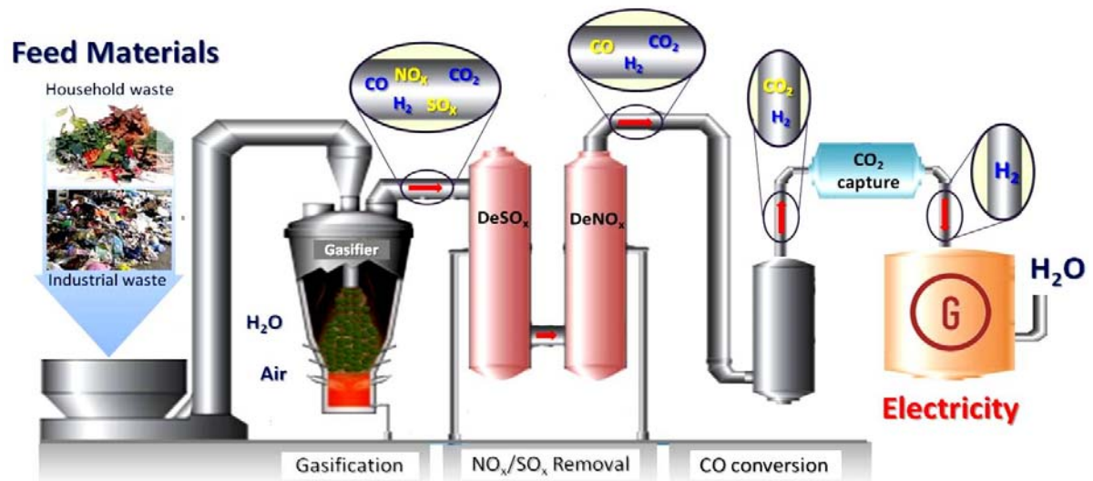
Figure 10: Basic schematic of gasification process and detail of gasification reactor
